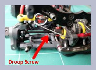
Measure at the bottom of the front steering blocks and the bottom of the rear hub carriers. Adjust the droop by turning the droop screws
